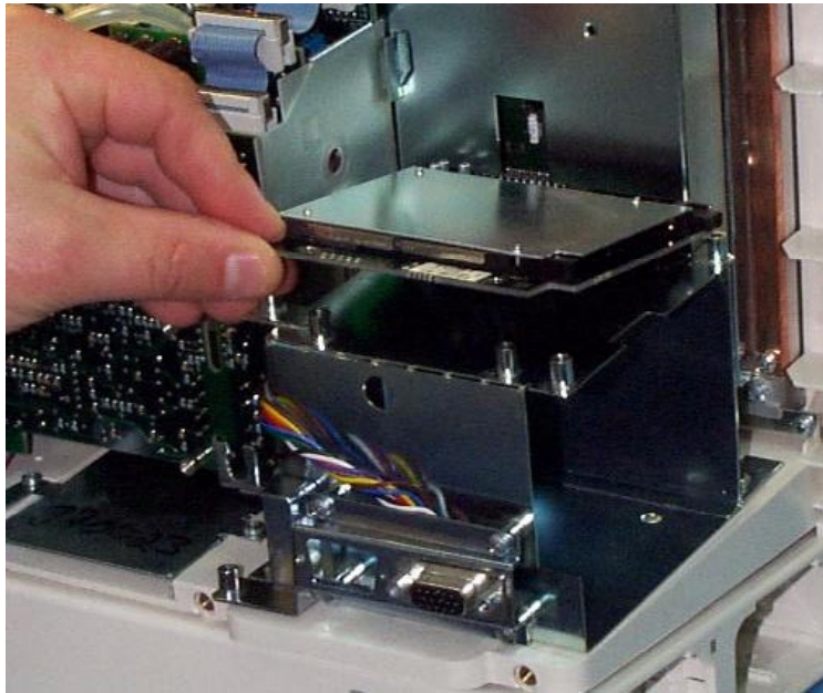
Figure 5 Lift the rear of the board before pushing the connector in
