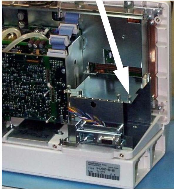
Figure 3 Data card hardware is installed on top of the recorder housing
