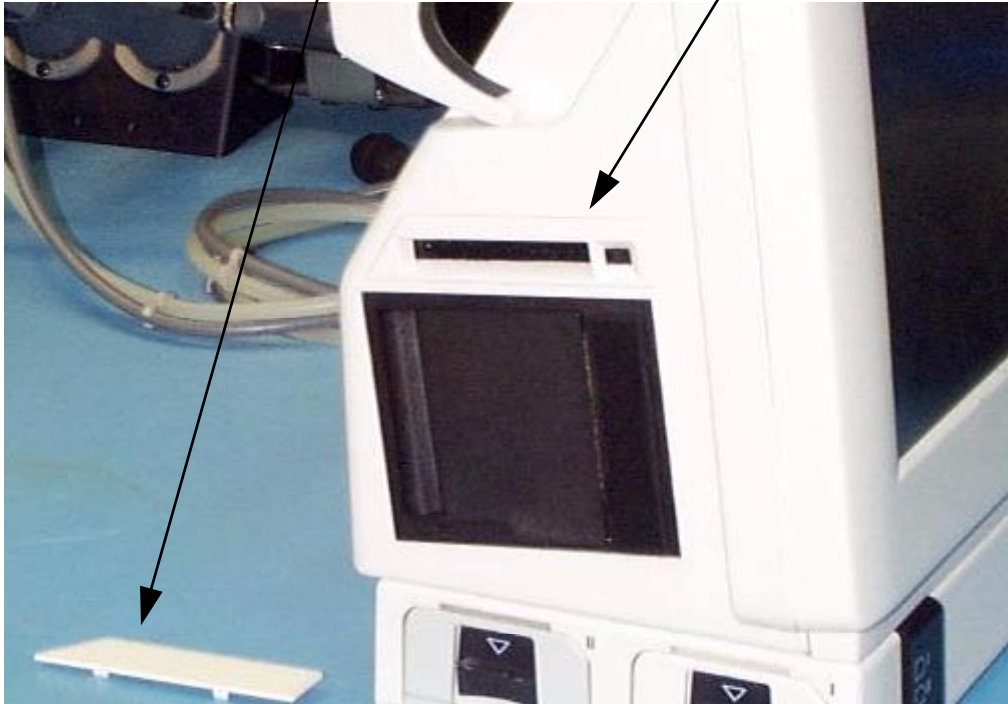
Figure 5 Replacing the cover plate
